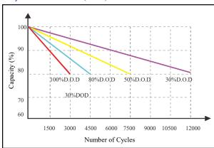
Note 2: The above curves are based on laboratory testing data @ 25°C 40%RH.
